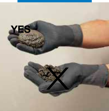
The correct consistency of Mapecem
